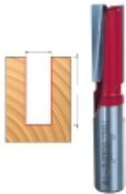
**Straight router bits:** A workshop staple, straight router bits make cuts straight into the mater to create a groove or dadoo (a groove across the wood grain) or to hollow out an area for a mortise or inlay. Straight bits come in a vast array of diameters and length.
