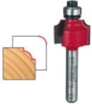
**Beading Router Bits** : Beading router bits are used for decorative purpose. They cut quarter-round shaped bounded by fillets. Beading router bits create a bead like contour on the wood piece.
